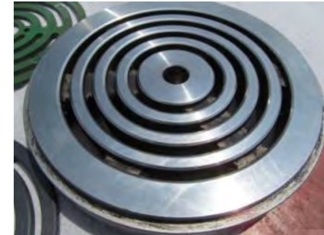
Valve Seat before & after hand clean up
