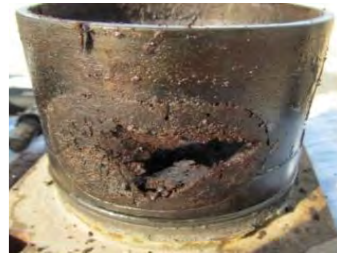
Retainer and valve with paraffin wax buildup
