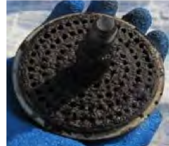
Retainer and valve with paraffin wax buildup
