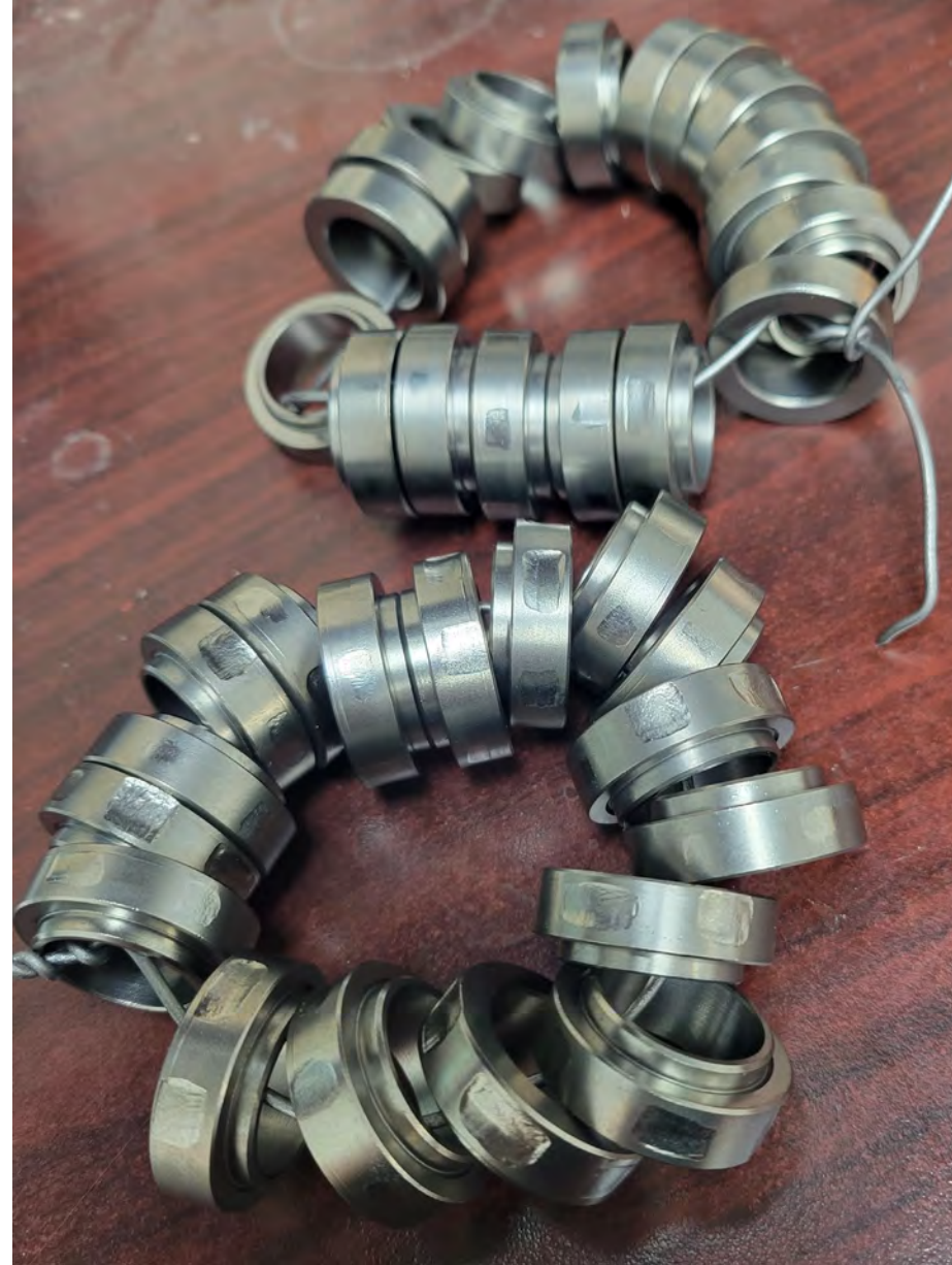
JGC/4 Compressor valve inspection after 5 years (approximately 40K hours)
