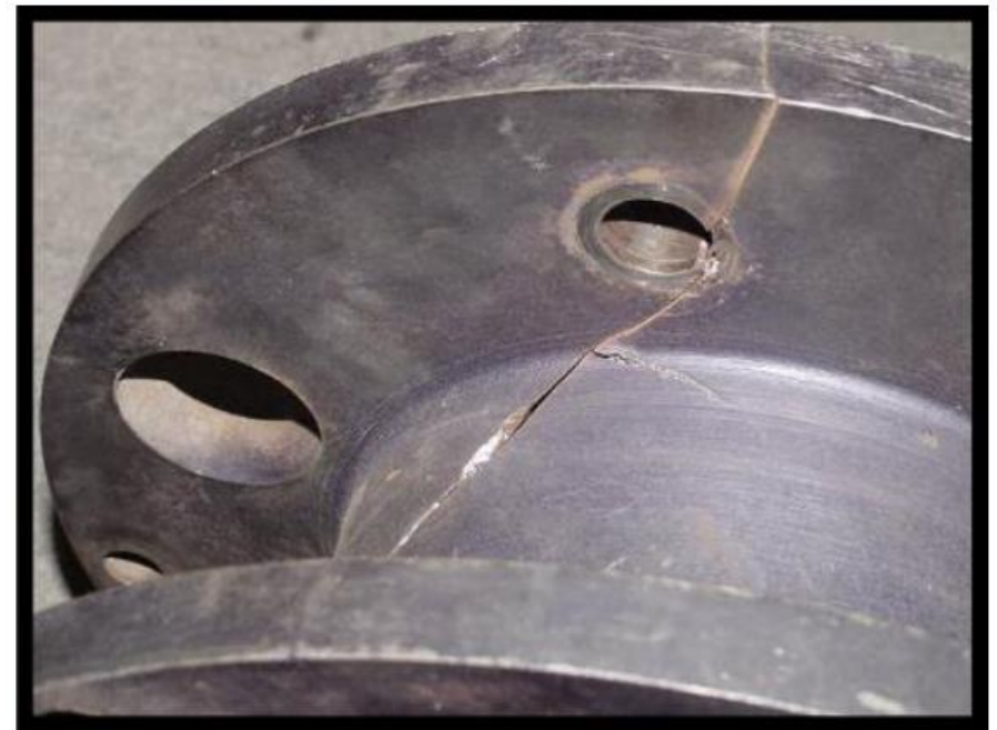
Coupling spacer with split crack due to high amplitude torsional vibration 3
