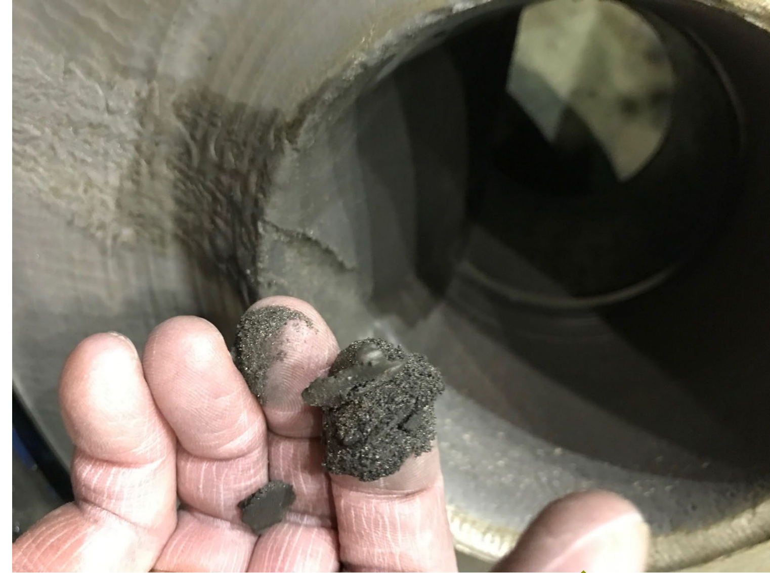
Tailings Slurry 3 to 4 times the sp.gravity of water. ↑
